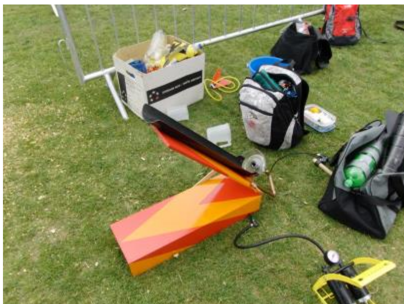
Bay 17: Compact launch rail with a modified Maplin launcher.
