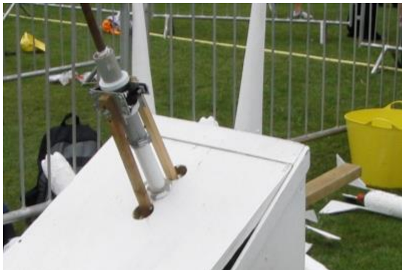
Brothers of Doom detail of launcher. The cable tie retainer is activated by a lever.
