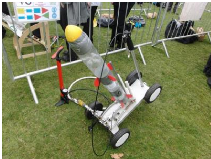
Bay 43: Rotating retainer allowing up to three simultaneous releases on portable trolley.
