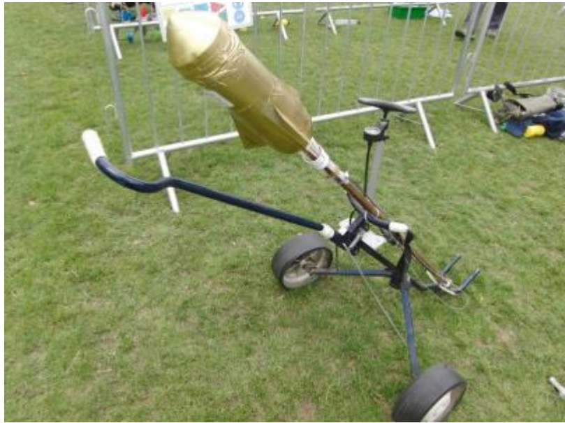
Bay 40: Cable tie launcher with launch tube based on golf trolley.
