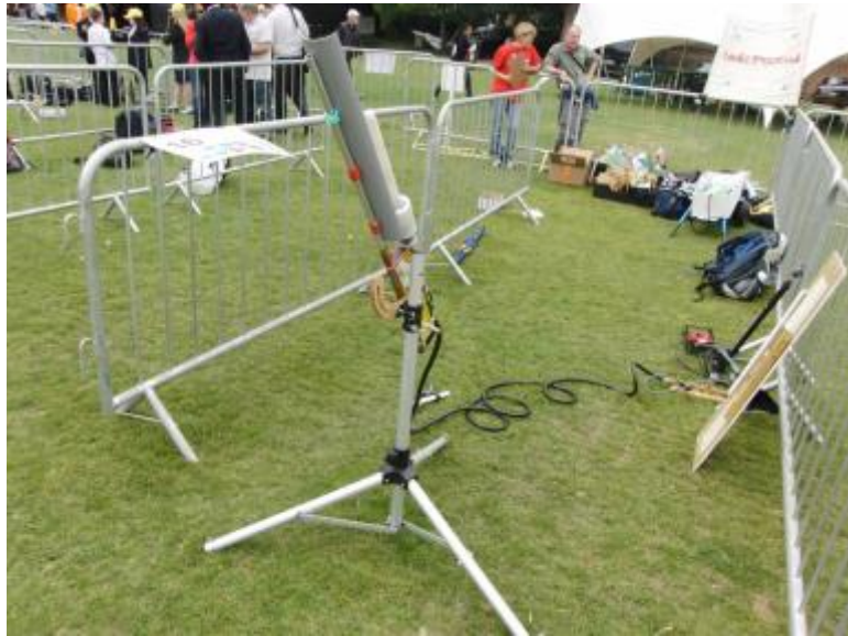
Bay 16: Cable tie launcher with launch tube and launch ramp held on a modified tripod.
