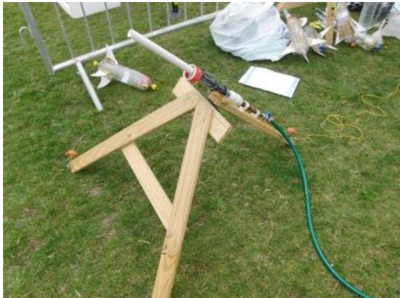
Bay 5: Cable tie launcher with launch tube on a frame.
