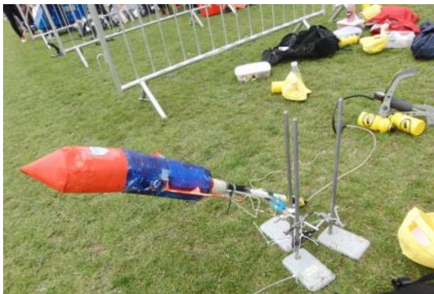
Bay 30: Cable tie launcher with launch tube and ad hoc clamp stand support.
