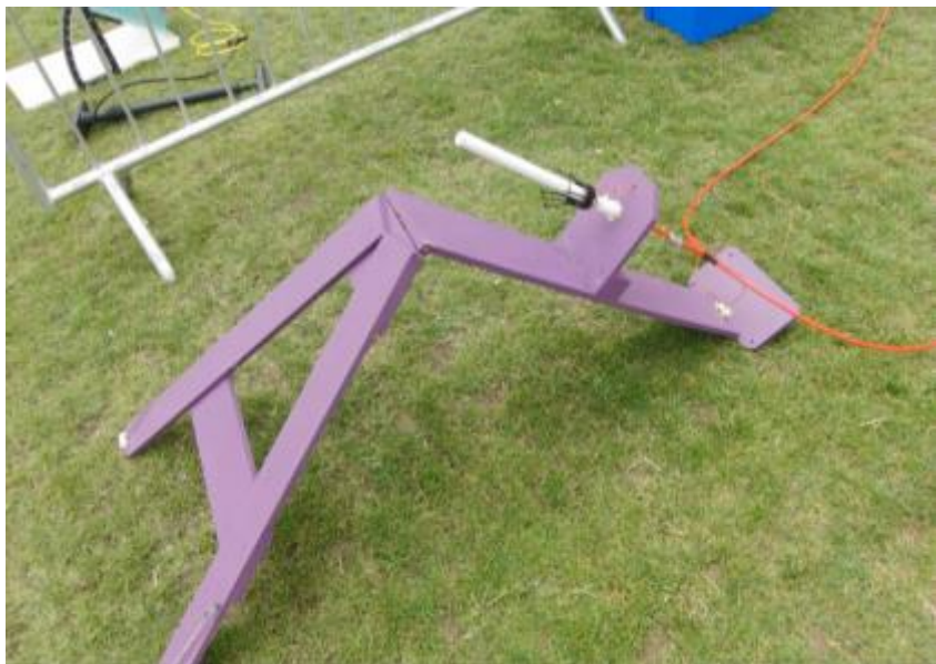
Bay 25: Cable tie launcher with launch tube on foldable frame.
