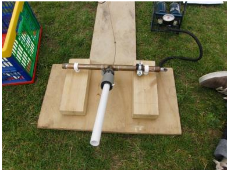
Bay 19: Cable tie launcher with launch tube.
