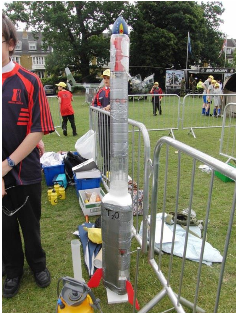
Bay 43: Rocket central part was made of custom formed plastic.
